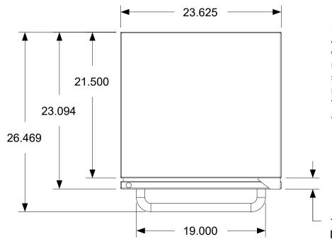
Dimensions shown are actual physical dimensions. Additional clearances to built-in cabinetry are dependent on the tolerances of the cut-out. We recommend an additional .250 inches around all side openings. An additional .500 inches is recommended for the top to allow for levelling of the fridge. Openings can be reduced if the tolerances are controlled.
